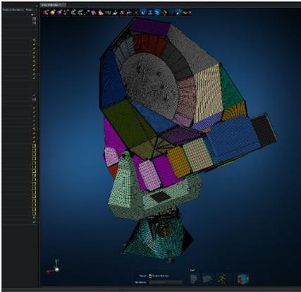
Apex's de-featuring functions easily simplified the massive parts of the telescope
