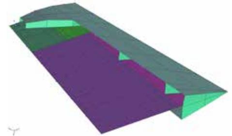
Splining of aerodynamic panel and structural mesh
