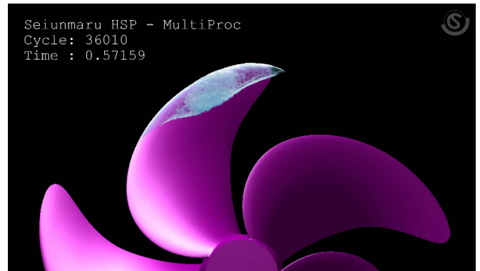
Cavitation generated around screw propeller (Volume rendered by bubble radius)
