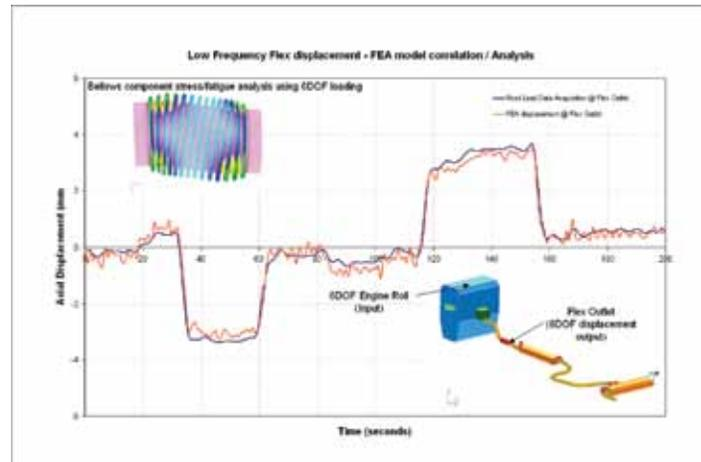
Validation of FEM model using Road Load Acquired Data
