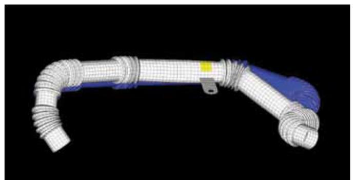
EGR pipe, mode and frequency analysis using the FEM
