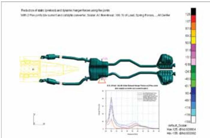
Reduction of static preload and dynamic hanger forces using flex joints in an exhaust system
