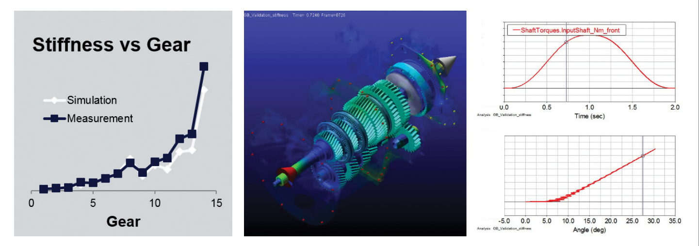
Excellent correlation between simulation and measurements in gearbox stiffness test
