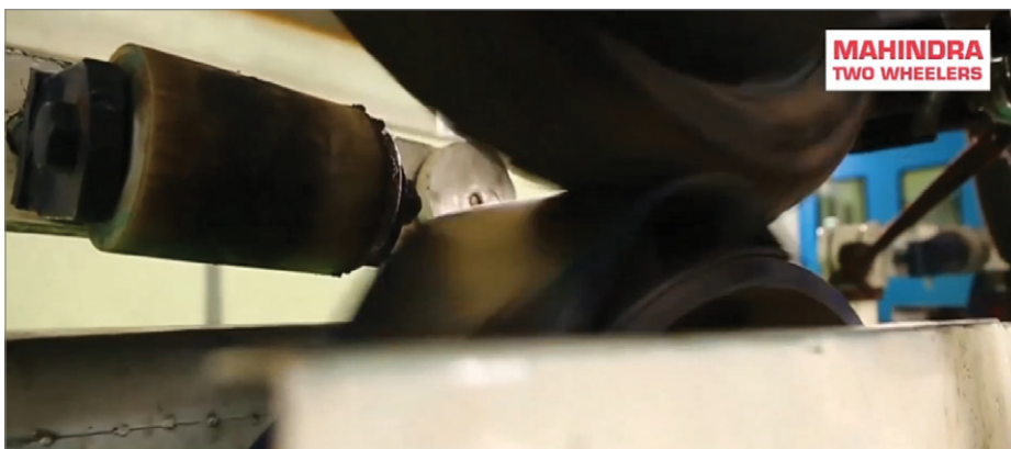
Bump rig test duplicates test track
