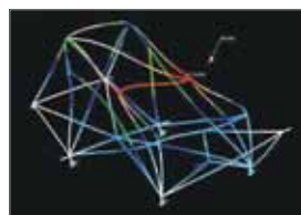
Integrated cage and shell design – simulation of lateral hoop test
